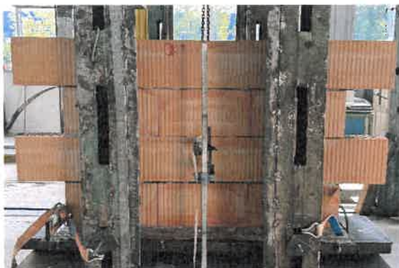
Figure 8 - Masonry specimen OK 1 prepared for test
