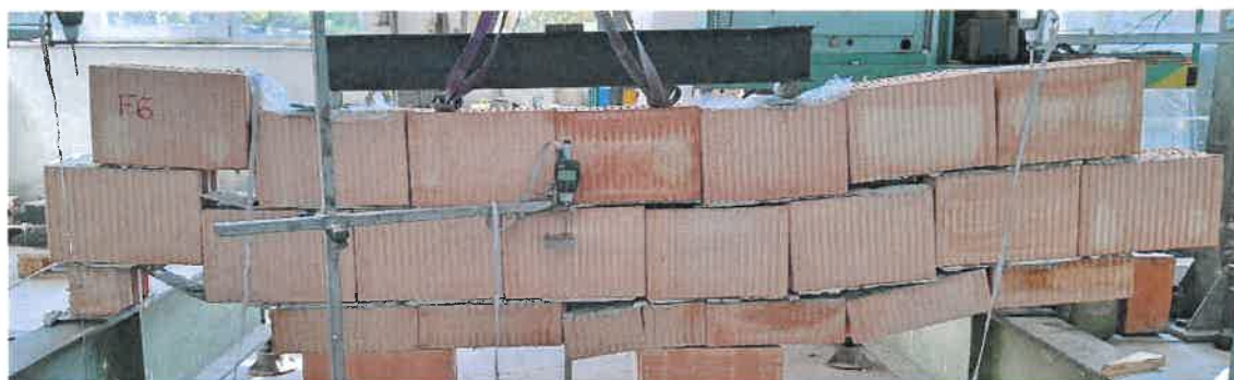
Figure 22 - Failure mode – F 6
