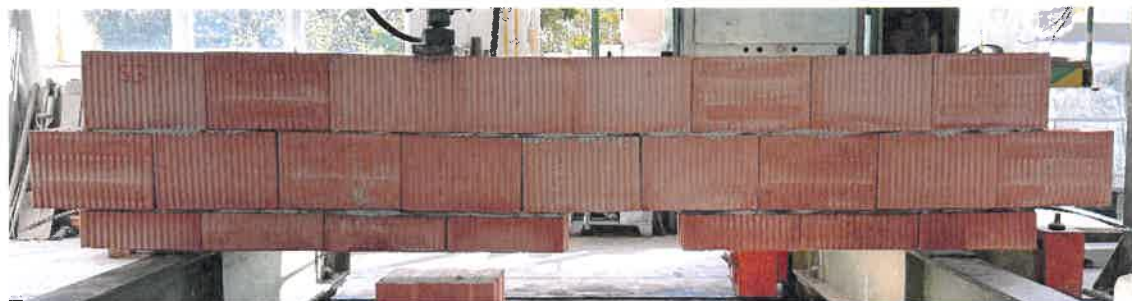
Figure 7 - First crack – S3
