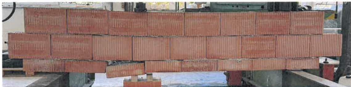
Figure 3 - First crack – S1
