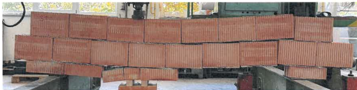
Figure 4 - Failure mode – S1
