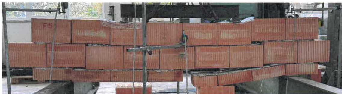
Figure 18 - Crack progress – F 5
