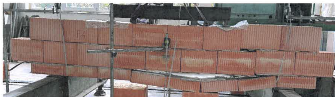
Figure 15 - Crack progress - F 4
